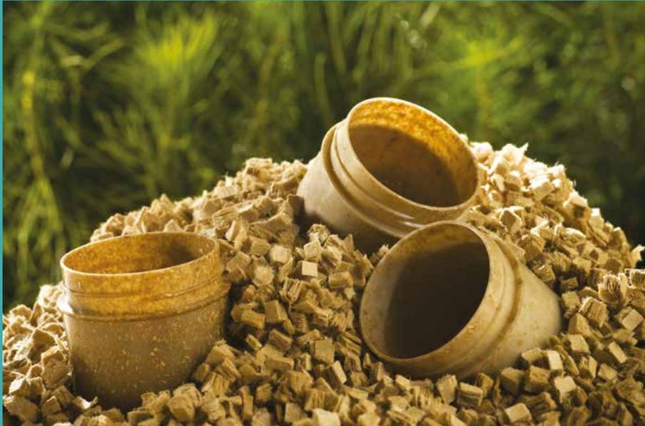
Bioplastic composites containing wood fibre. Photo: Scion.
